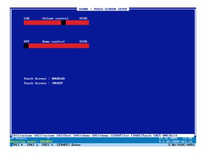
Exit the submenu by pressing the BET button. Go to the EXIT menu by means of Hold1 and press START twice to save the settings and to exit the service menus. The program will reload.
