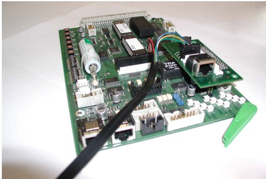
Figure 3: Connecting the Cash Fever™ PC to the Commboard
