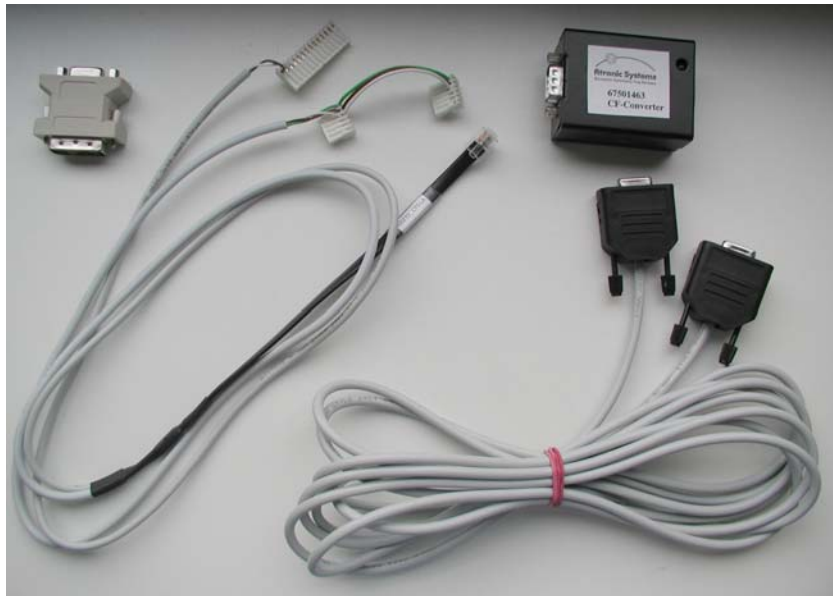
Figure 2: Cash Fever™ connection kit - adapter, converter and cables
