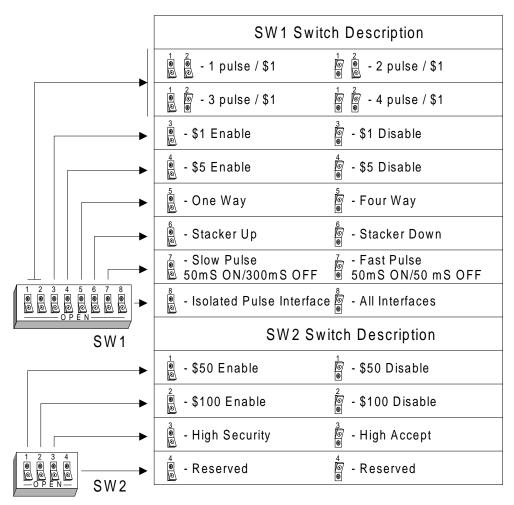
Each switch is assigned to control the settings shown below.
