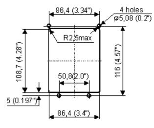
The figure «Layout Of Mounting Holes» shows the template for panel of the external equipment where the Bill Validator is to be mounted. All the dimensions are in millimetres and inches (in parenthesis).
