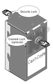
□ The Bill Validator stacks accepted banknotes into a high security lockable and removable cassette (LRC). The design of the Cassette guarantees reliable protection against unauthorised access to its contents.
