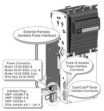
2. When used in the external equipment supporting Isolated Pulse Interface, the Bill Validator is to be connected with the 6 Pin Power Harness PT# OPT-HS-12v-06p; and the Jumper Connector PT# OPT-HS-JC18 may be applied to the 18 pin interface connector of the Bill Validator if required.
