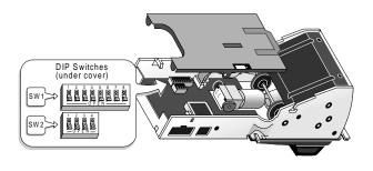
To change the position of a DIP switch, use the point of a sharp instrument.
