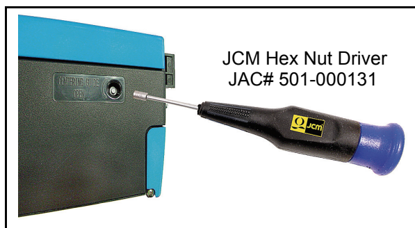
Figure 2-17 Opening UBA Centering Mechanism
